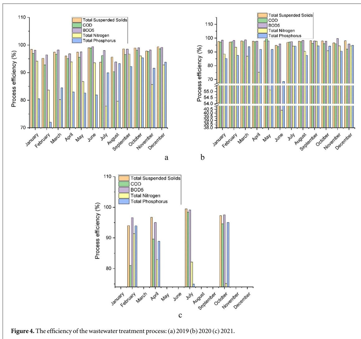
Figure 4. The efficiency of the wastewater treatment process: (a) 2019 (b) 2020 (c) 2021.
