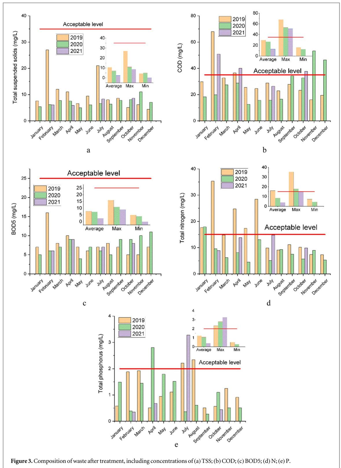
Figure 3. Composition of waste after treatment, including concentrations of (a) TSS; (b) COD; (c) BOD5; (d) N; (e) P.
