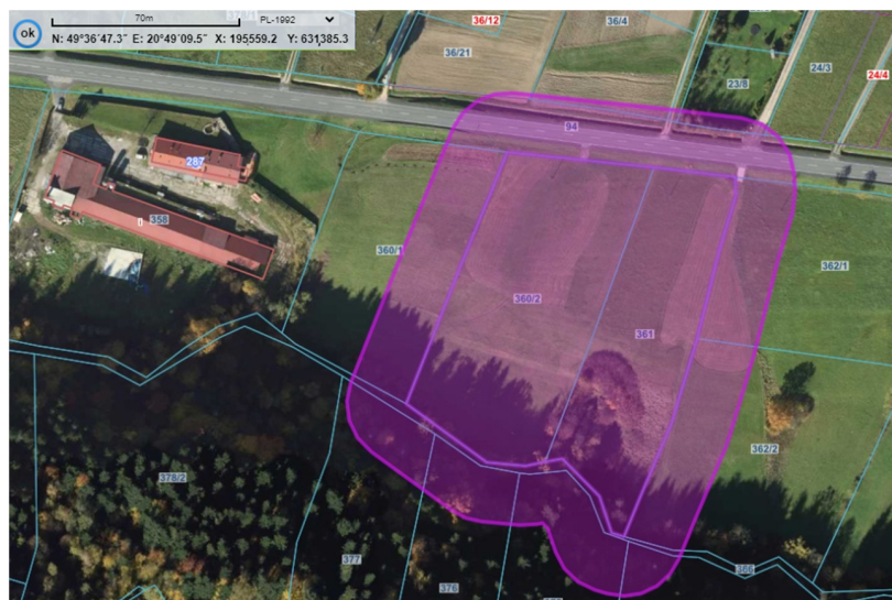
Figure 8. An extract from an orthophoto showing an example of a distance buffer (purple area) of 25 m imposed by law [101].
