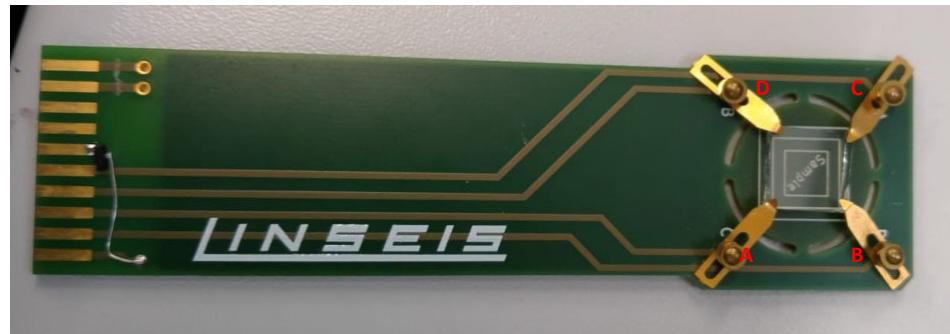
Figure 1. A sample with dimensions of 10 × 10 mm 2 was mounted in the sample holder.
