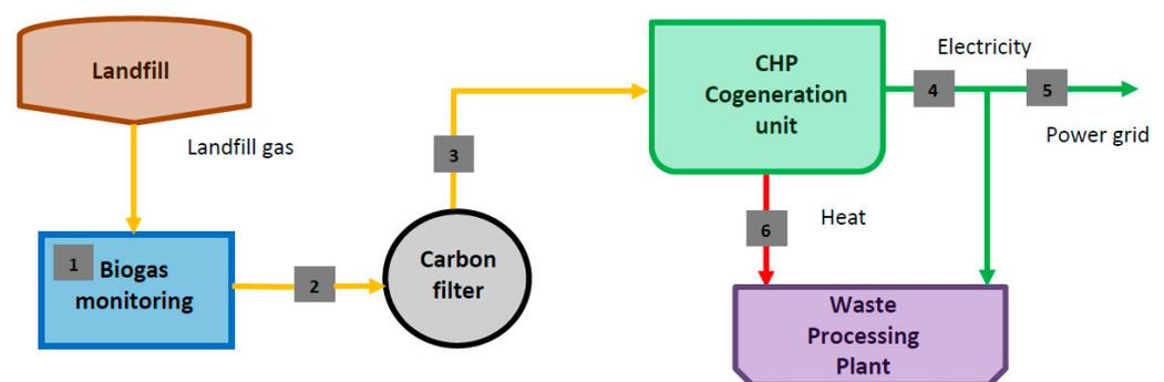
**Figure 1.** Installation of biogas energy utilization at the landfill.
