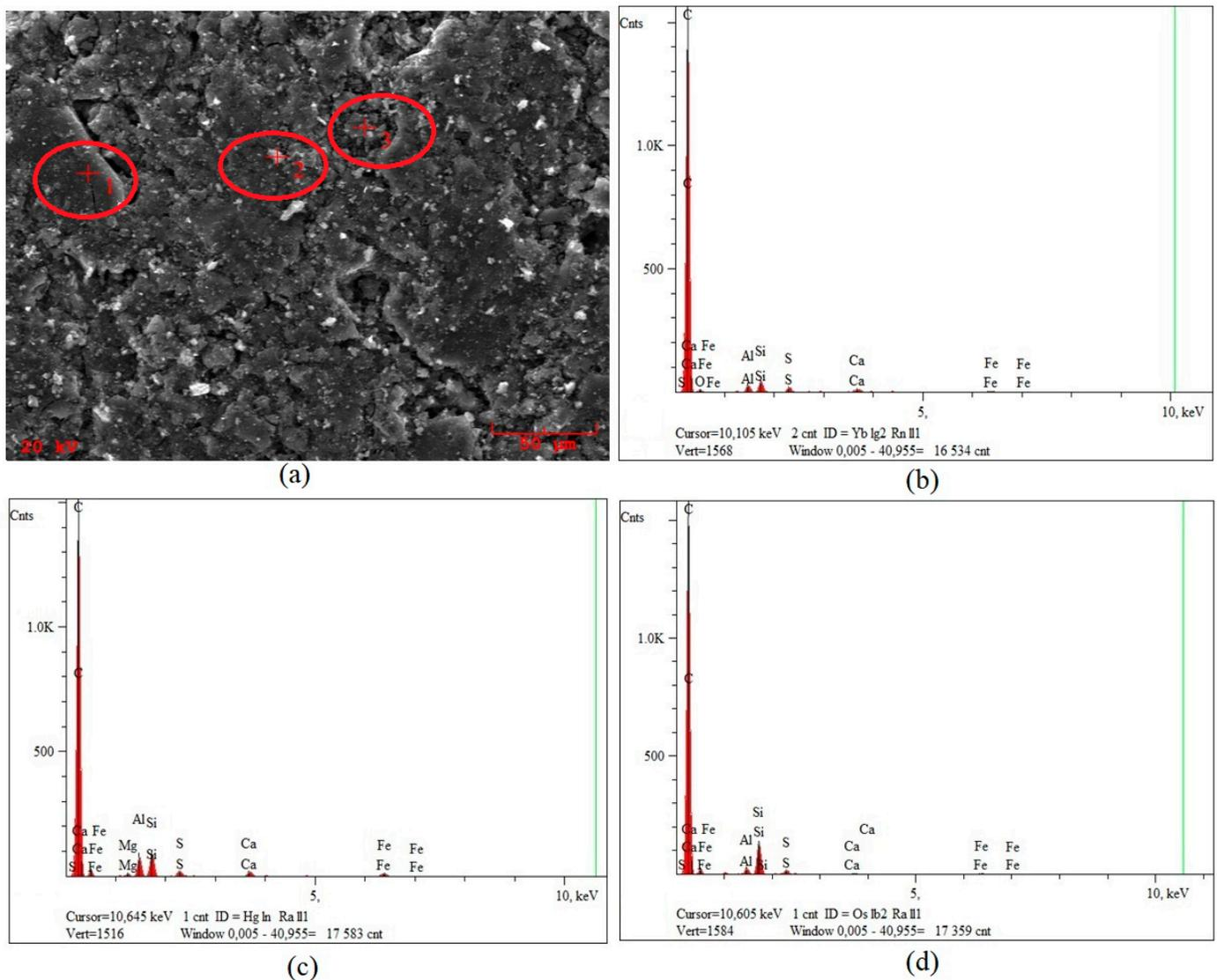
**Figure 4.** Scanning analysis of activated carbon: (a) SEM microscopic image; (b–d) chemical composition of points 1, 2, 3.
