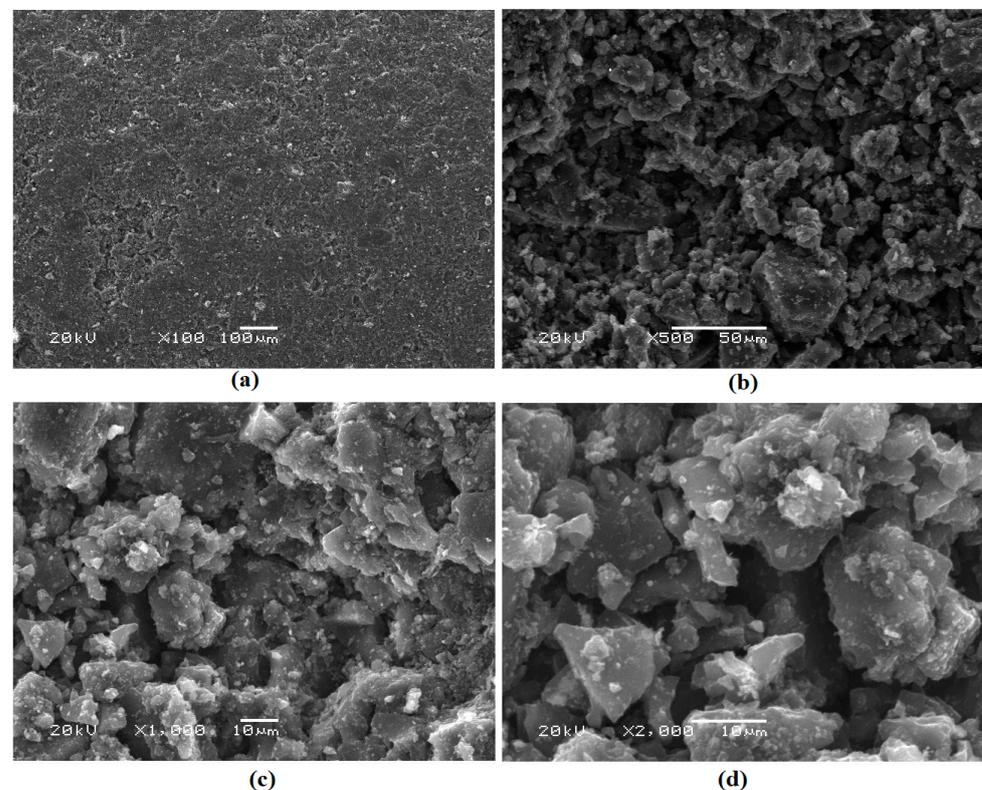
**Figure 3.** Images of the surface state of the new activated carbon under appropriate magnification: (a) 100; (b) 500; (c) 1000; (d) 2000 times.
