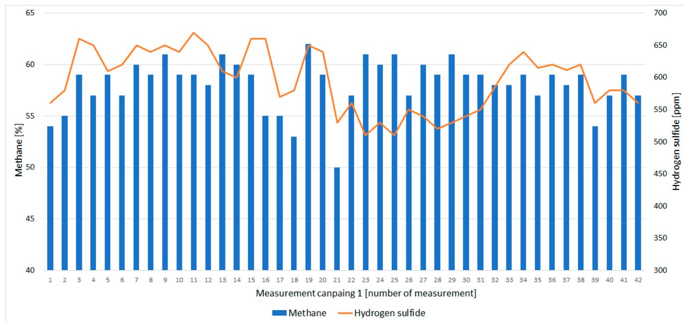
**Figure 2.** Methane and hydrogen sulfide parameters for “raw” untreated gas.
