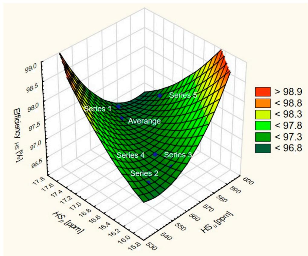
**Figure 8.** Efficiency of hydrogen sulfide removal depending on its content.
