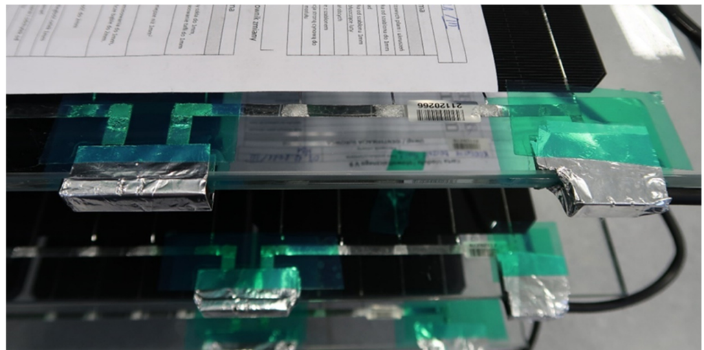
Figure 3. Connectors covered with aluminum foil to ensure proper electrical contact with the tested connector surface.
