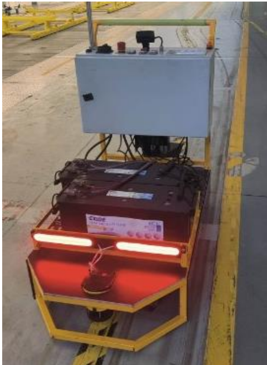
Figure 11. Traffic lights showing the status of the AGV (technological audit). Source: own study based on a technological audit of the FCA car assembly hall.
