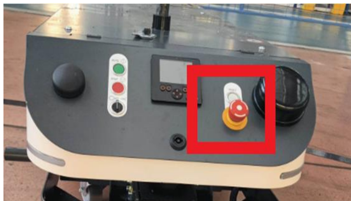
Figure 10. Main safety switch on the AGV (technological audit). Source: own study based on a technological audit of the FCA car assembly hall.
