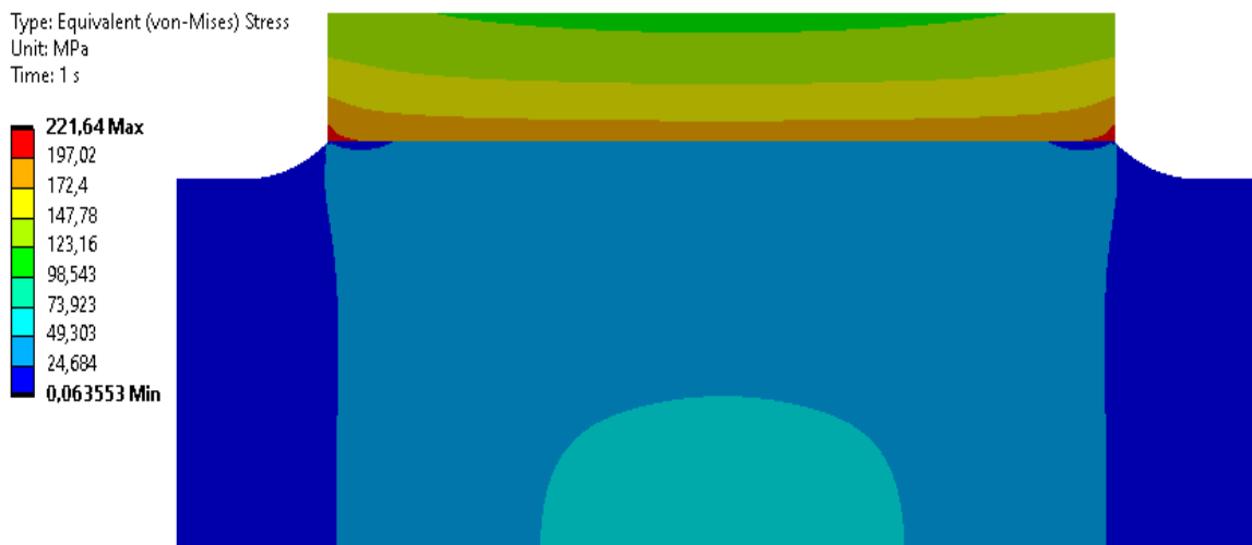
Figure 11. Stress distribution in the longitudinal section of an interference fit connection variant W00. Source: own elaboration.
