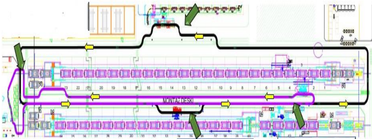
Figure 2. Lay-out of a fragment of a car assembly line with marked combined AGV routes (technological audit)
