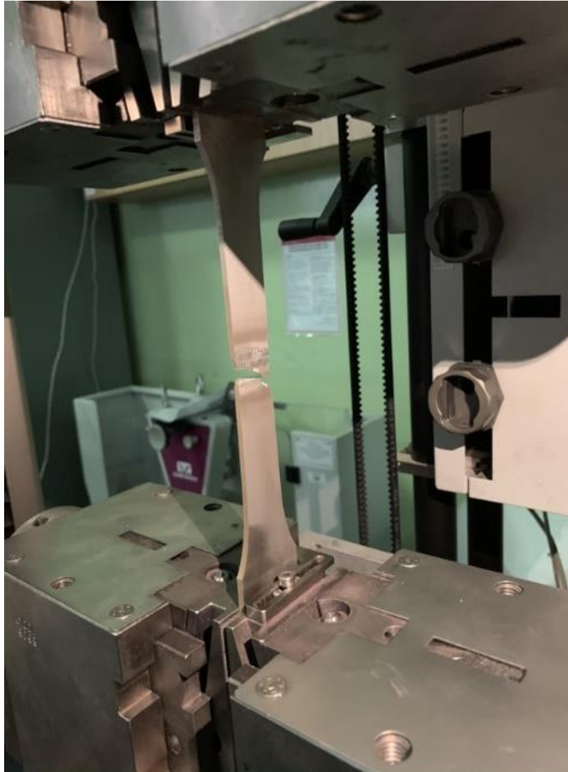
Figure 5. Sample mounted on Zwick/Roell Z 100 ripper. View after rupture. Source: own elaboration.
