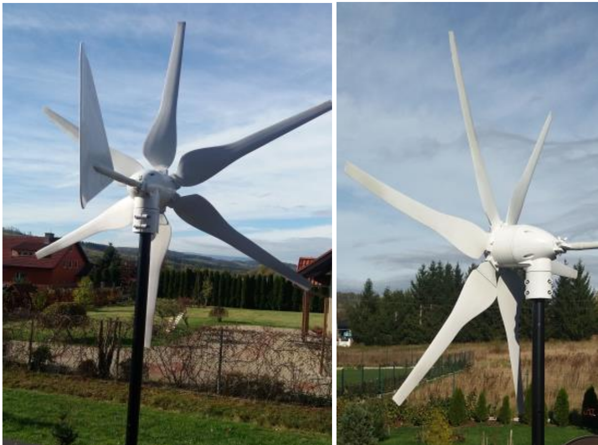
Figure 10. Wind turbine mounted on a test stand. Source: own source.
