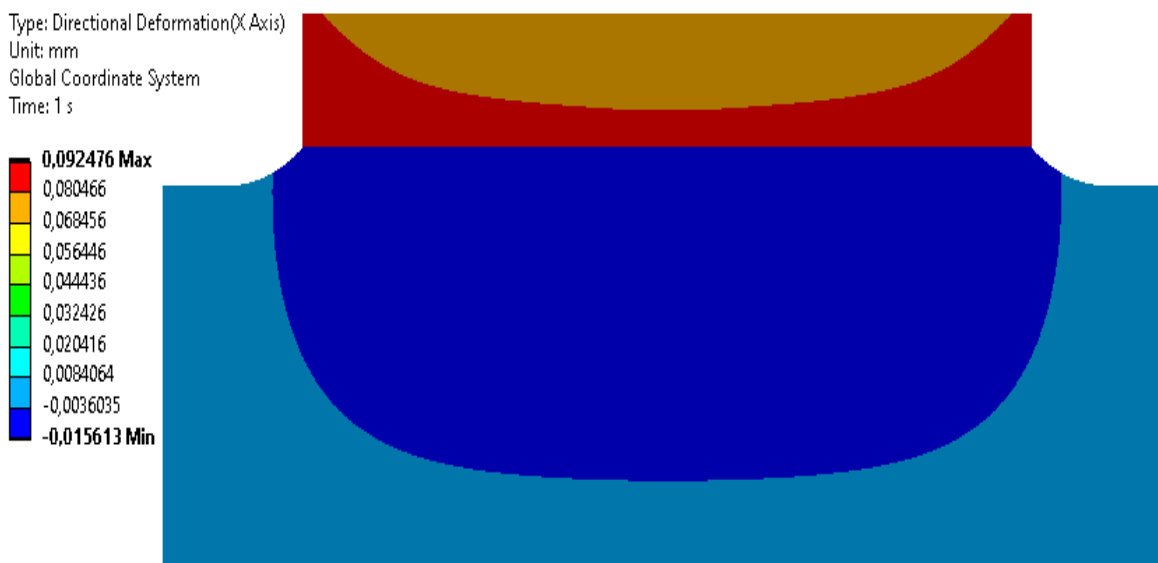
Figure 12. Stress distribution in the longitudinal section of an interference fit connection variant W00. Source: own elaboration.
