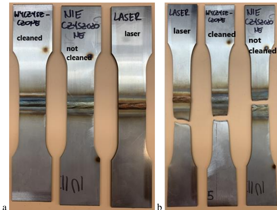
Figure 4. Views of samples used in static tensile testing, (a) pre-rupture view of samples, (b) post-rupture view of samples. Source: own elaboration.
