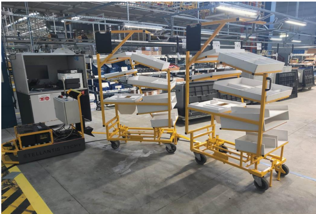
Figure 8. AGV trolley with trolleys transporting small assembly elements (technological audit). Source: own study based on a technological audit of the FCA car assembly hall.
