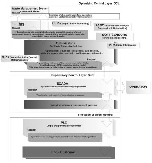
Fig. 2. Architecture/Topology of the System
