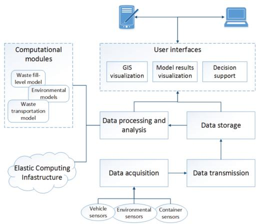
Fig. 1. The Topology of the Expert System
