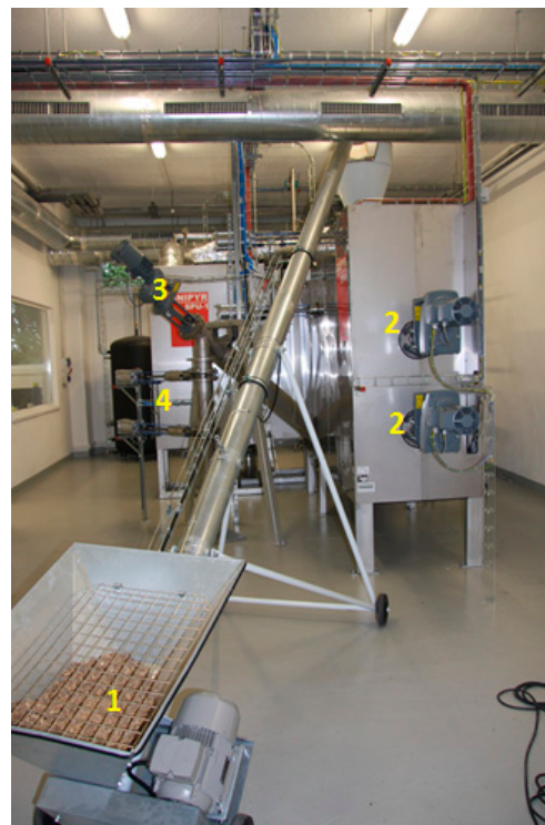
Figure 3. Assembly of the pyrolysis unit. 1—biomass conveyor, 2—reactor, 3—carbon conveyor, 4—condenser.
