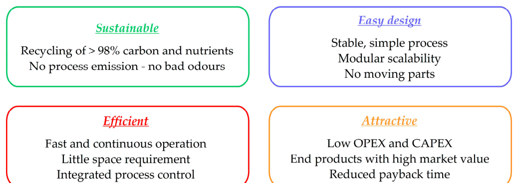
Figure 5. Advantages of the Ingelia hydrothermal carbonisation process.
