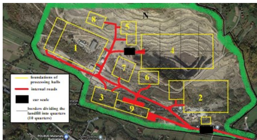
Figure 4. Layout of buildings and facilities of the planned Waste Management Plant in the Sądecki Subregion
