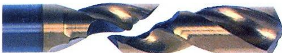
Figure 4. Fracture on the cut of the helical drill. Source: own study.
