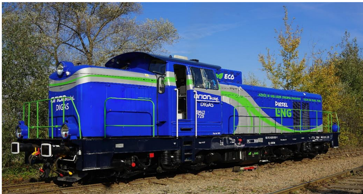
Figure 1. SM 42 locomotive in a dual-fuel system – Garodiesel.
