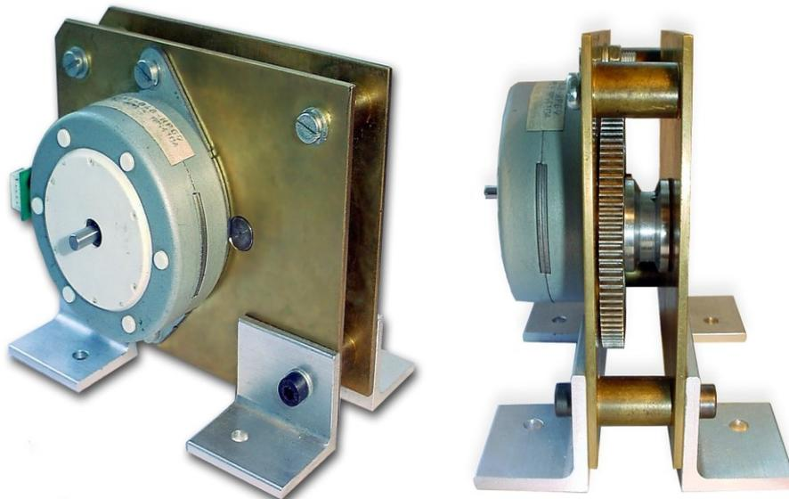
Figure 11. The prototype of stepper-motor module for controlling the valves in the tone windchest
