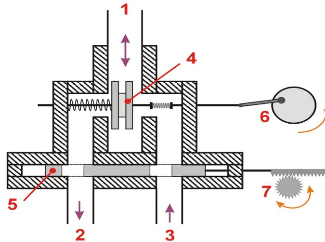
Figure 10. Tremulant construction scheme with adjustable amplitude and frequency
