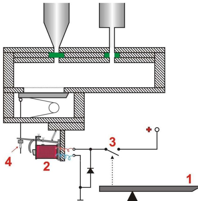
Figure 8. Scheme of electromagnetic key action in conjunction with pallet windchest
