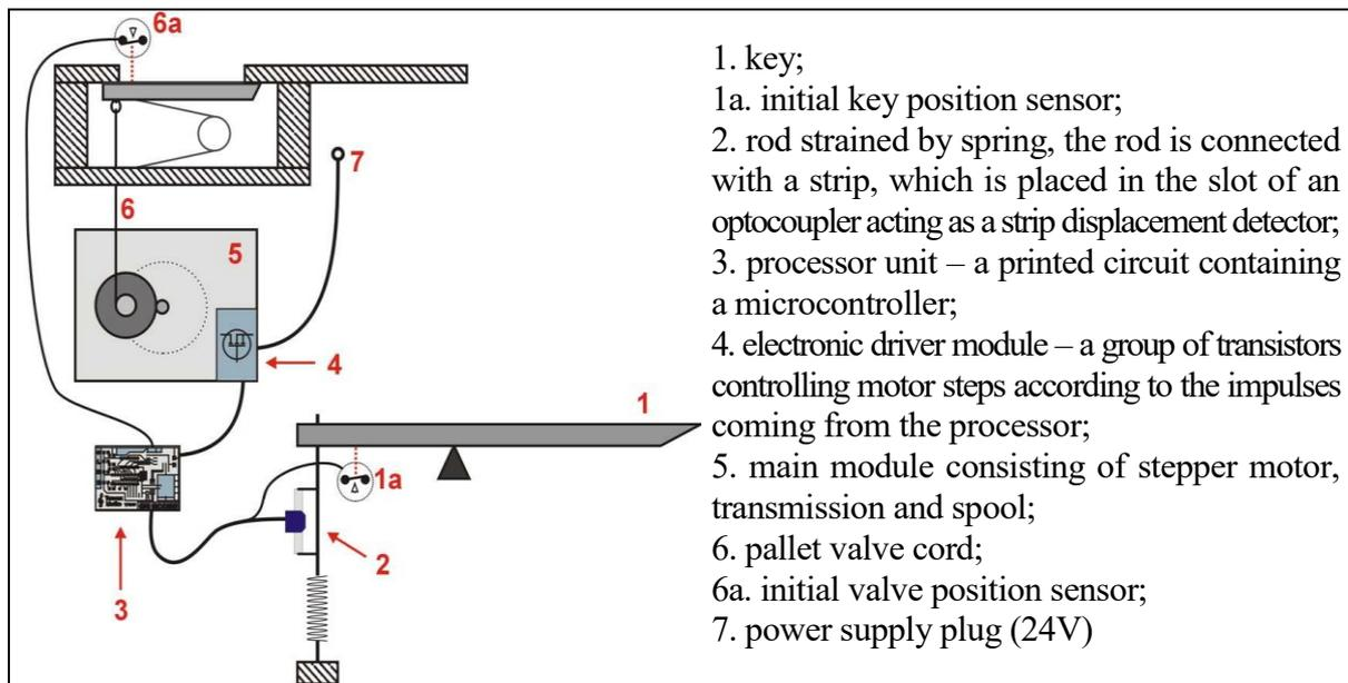
Figure 13. Mechatronic tracker action – schematic diagram
