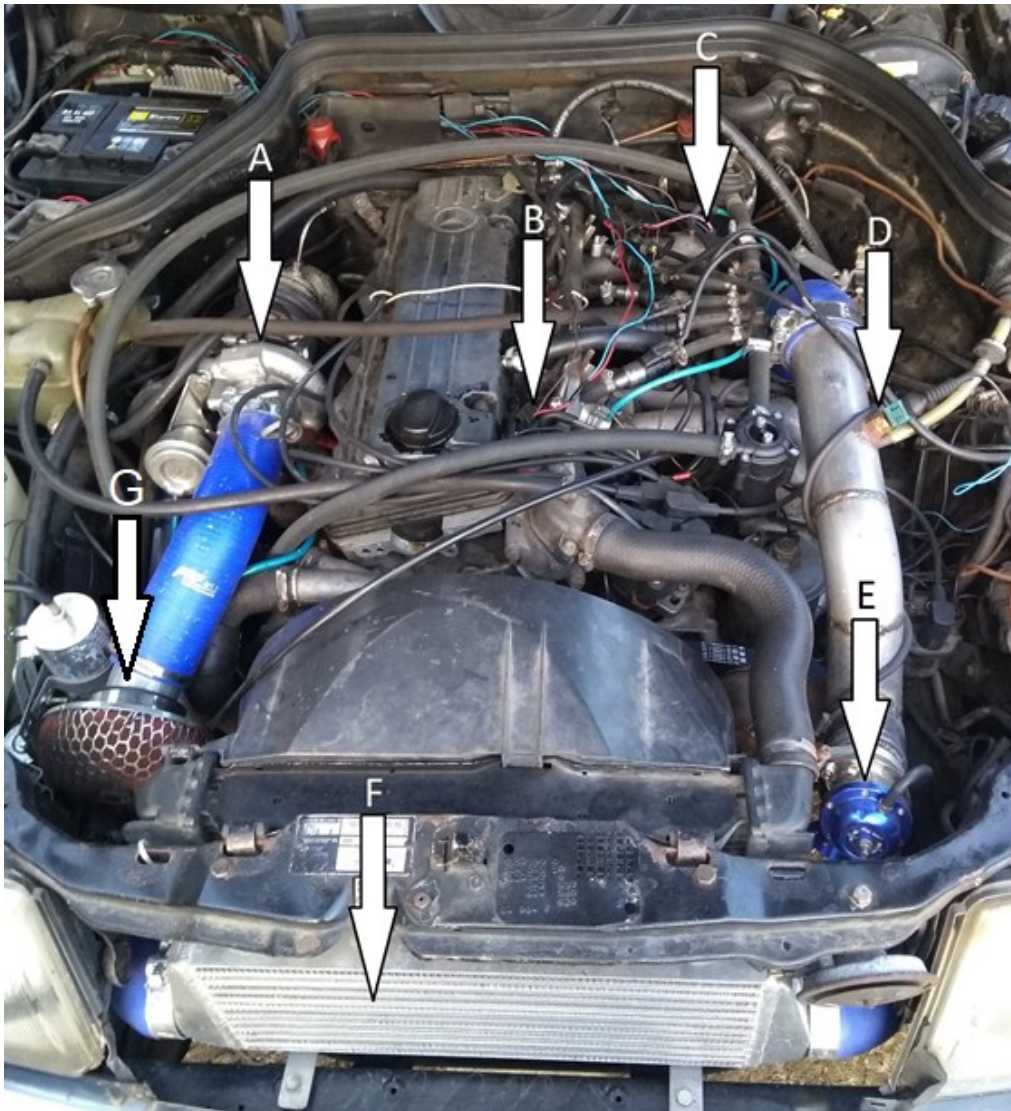
Figure 5. View of the engine with modifications and location of measuring transducers indicated A – turbocharger, B – cooling liquid temperature transducer, C – intake pressure transducer, D – intake air temperature transducer, E – air bleed valve, F – air cooler (Intercooler), G – cone filter
